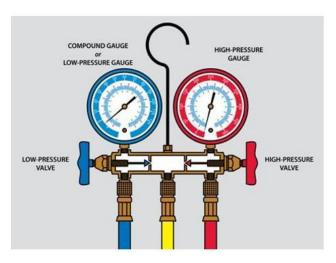
The compound gauge measures low pressure (psig) and vacuum (inches Hg.). The highpressure gauge measures high side (discharge) pressure.
