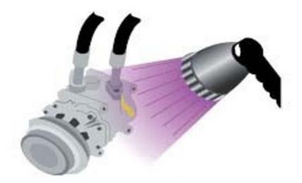
UV- Lamp Leak Detection
