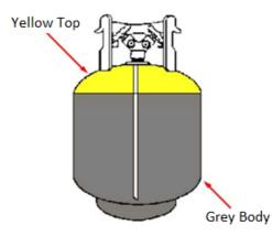
It is important to ensure that the recovery cylinder is only ever used for one type of refrigerant. This rule should be followed for two reasons: first, if different refrigerants are mixed, it may not be possible to separate them again for re-used, and secondly, mixing two or more refrigerants can result in a pressure that exceeds the pressure of either of the refrigerants added into the cylinder.
