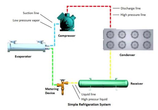
Let's look at what happens in a simple refrigeration cycle, and to the major components involved. Two different pressures exist in the cycle - the evaporating or low pressure in the "low side," and the condensing, or high pressure, in the "high side." These pressure areas are separated by two dividing points: one is the metering device where the refrigerant flow is controlled, and the other is at the compressor, where vapor is compressed.
