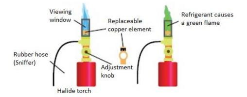
Halide Torch Leak Detection
