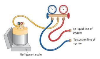
Setup for Passive Refrigerant Recovery
